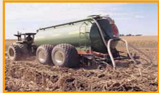
Liquid Slurry Tank System Equipped with an Injection Toolbar
